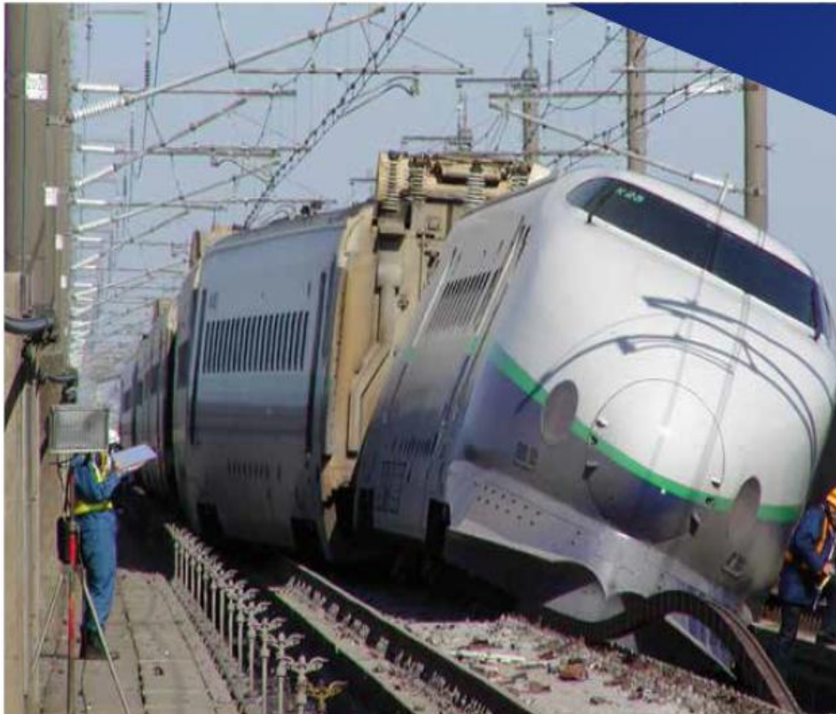
Image 1: A derailed Shinkansen bullet train, Niigata Prefecture, Japan, 2004. Source: Japanese Transportation Safety Committee.
